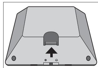
*Press firmly on the snap hook to remove the back cover.*
