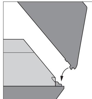
*Make sure to align the pivot points at the edges before closing the back cover.*
